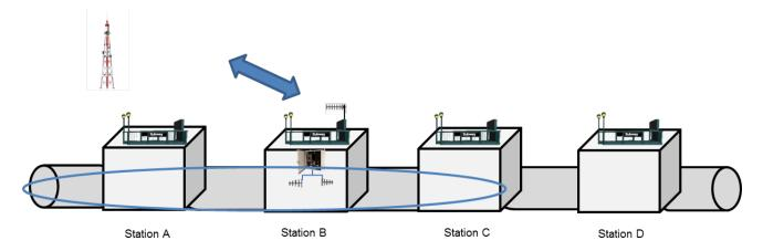
Diagram 1: Tunnel coverage from one DVRS on located at station B – Using 1 Frequency
