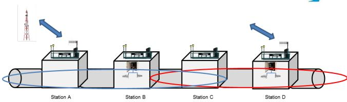
Diagram 2: Tunnel coverage from two FDVRs located at station B & D – Using 2 Frequencies
