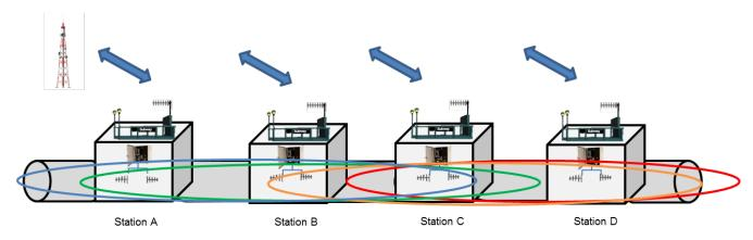
Diagram 3: Tunnel coverage from four FDVRs located at each station Using 4 Frequencies
