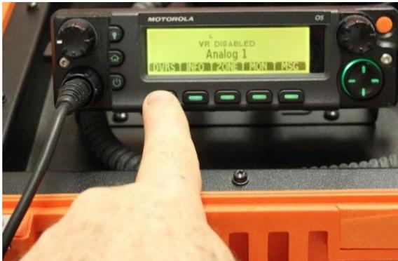
The DVR/VRX1000 connects directly to the APX mobile radio and essentially becomes part of that mobile radio. The APX mobile continues to operate while the DVR/VRX1000 is active. All control of the DVR/VRX1000 is achieved through the mobile control head and DVR/VRX1000 status is displayed on the mobile control head. This status includes: channel, mode, TX/RX and primary/secondary state.
