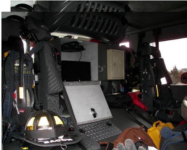
*DVRS Installed in Protected Box in Pumper Cab*
