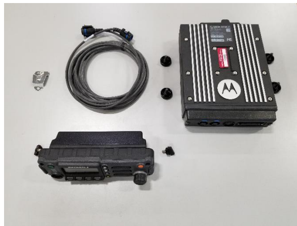
Figure 4 - MSU parts to be installed in the tray (The Microphone is installed on the front panel)
