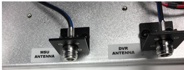
Figure 13 - MSU (System) and DVR (Local) Antenna connector location
