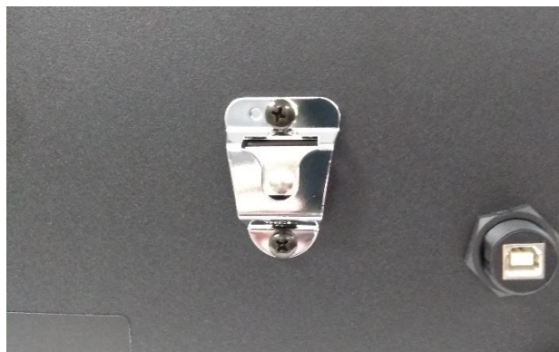
Figure 8 - Installation of the microphone clip
