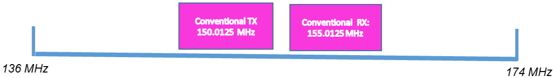
Figure 13 – Conventional VHF System Frequencies
