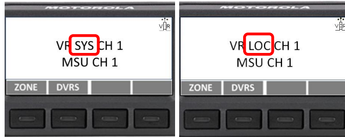
Figure 7: Control Head Display--System/Local
