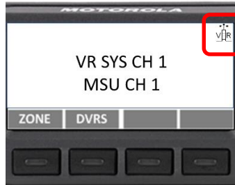
Figure 5: Control Head Display--Status Icon
