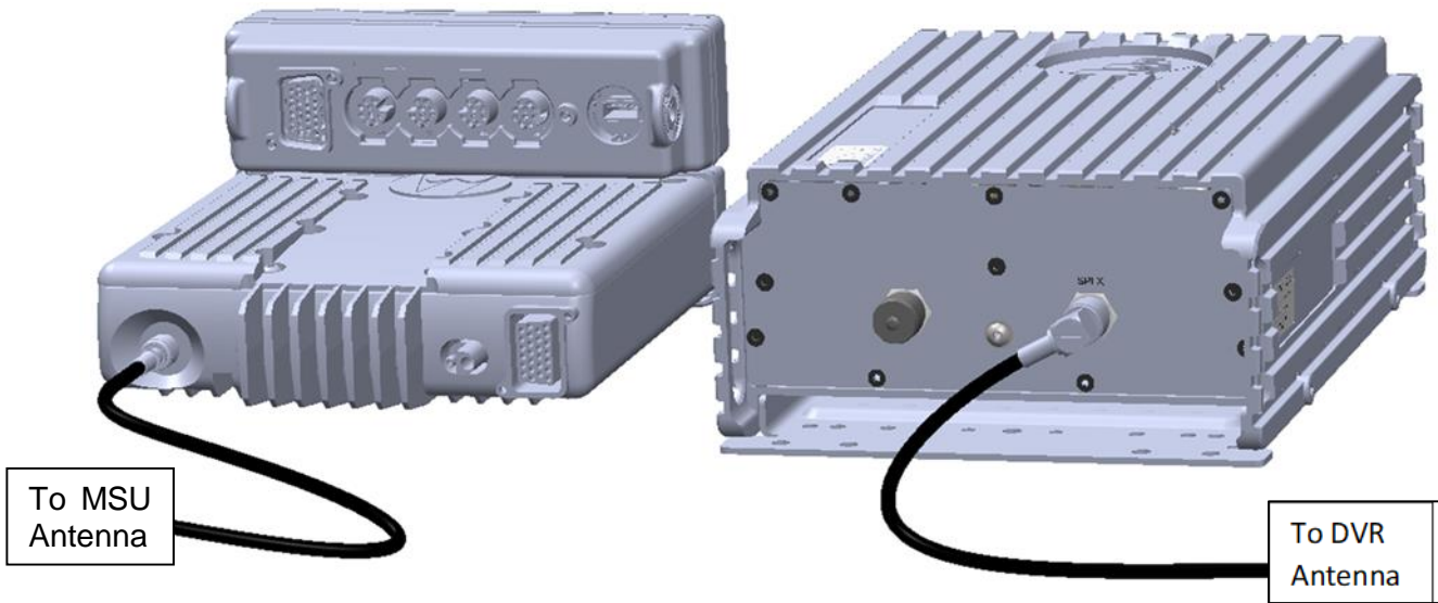
Figure 24: DVR-LX Cross-Band Simplex (Back)
