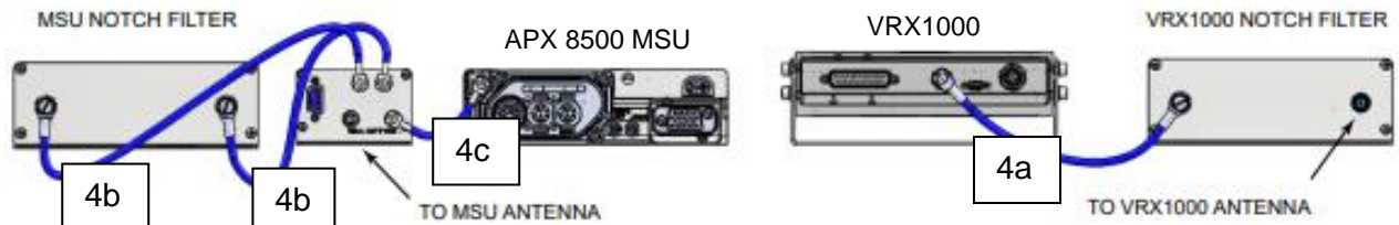
Figure 26: Configuration 4--Back View (Connection Cables for Filters, RF Switch and Antenna Ports)
